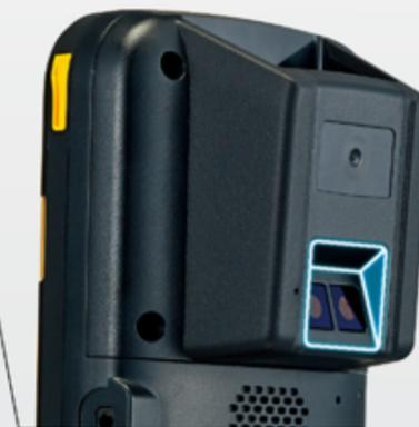
Optional 13 MP camera embedded with specific angle to prevent it from being blocked by user's hand while gripping pistol or taking photos.
