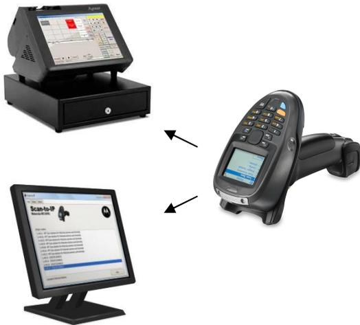
Truck terminals with a MT2090 WLAN scanner connected. Pair only by scanning the truck terminal's ID (IP), or change the pairing by scanning another terminal ID.
