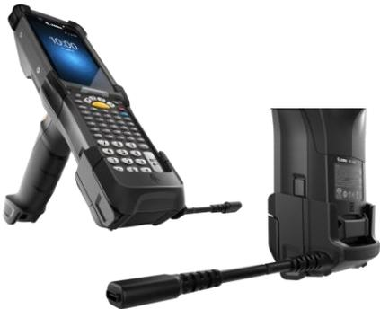
**CBL-MC93-USBCHG-01:** USB cable, provides fast-charge when a MC93 PP+ battery and a wall adapter is used, it also allows USB communication to the device when connected to a PC.
